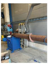
Photo: Screw for discharging cutter shavings produced in the maintenance department with a welding jig developed in-house.
